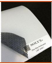
SOLYX® **SX-1940 One Way Perforated** film is designed for exterior window applications. The design of the black/white PVC material allows for one-way display applications and shading. White on print side and black on adhesive side. Manufactured with a silicone paper liner, which protects the clear, pressure-sensitive adhesive, and applied using the same tools and techniques for window films.
